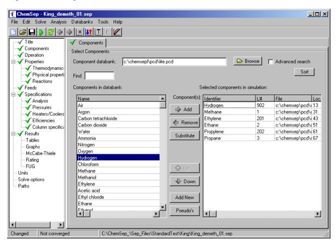
This is the part of *ChemSep* where we add and subtract components to be used in the simulation. In what follows we describe how to use this panel.
